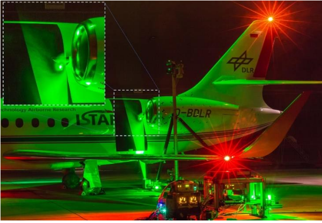
Figure 7: Full scale engine flow field measurements applying stereoscopic PIV at different measurement planes (detail = inlet vortex in front of the engine).
