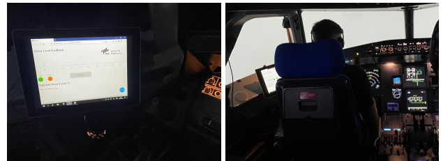
FIG 5. Integration of the OSAT inside the AVES A320 flight deck. left: close-up of the captain-side tablet.
