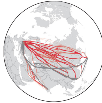
FIG 13. The trajectories of the German airlines Aerologic and Lufthansa Cargo operating a single O/D pair in 2019 (red) and 2022 (black distribution) (own figure).
