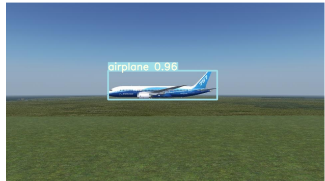
FIG 1. Detection of an object of the class "airplane" represented by a bounding box.
