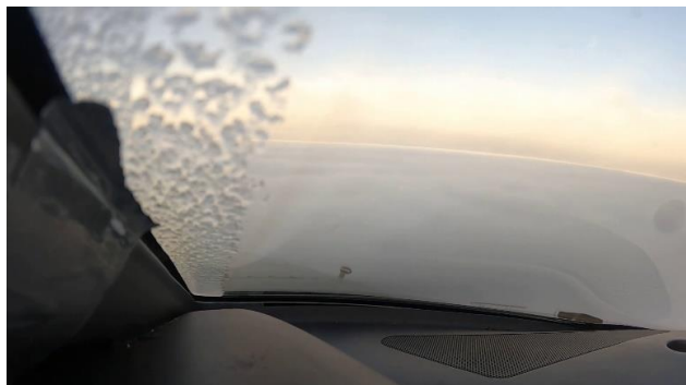
FIG 10 Ice accreted on Phenom 300 windshield after leaving clouds with supercooled liquid water [image Embraer]
