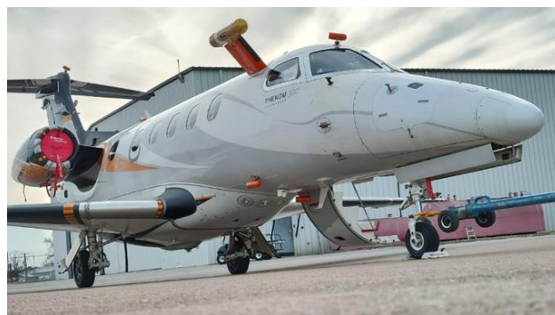
FIG 8 Embraer Phenom 300 with test sensors and reference instruments [image Embraer]
