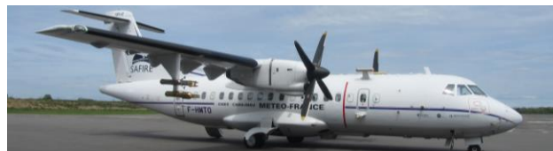
FIG 11 SAFIRE ATR 42 with test sensors and reference instruments [image DLR]
