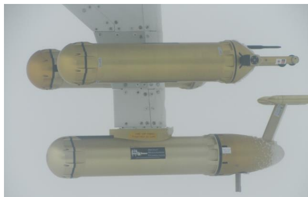
FIG 7 DLR and Safire instruments installed on Safire's ATR-42 with ice accretion on the unheated parts while inside supercooled liquid clouds [image DLR]
