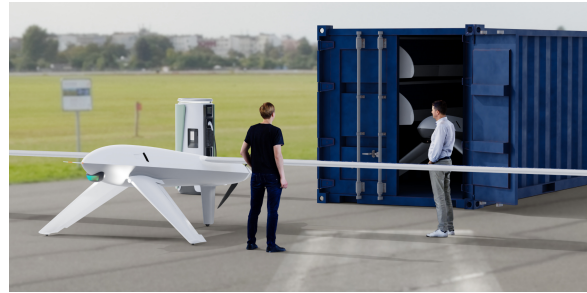
FIG 21. Conceptual visualization of HEIKE 's airfield-based charging equipment and transportation container
