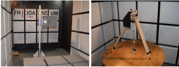
FIG 8. Reference Antenna Schwarzbeck BBHA9120E (right) and AUT LD-Systems WS 100 DA (left)
