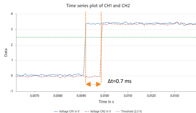
FIGURE 2. Exemplary plot of data obtained from oscilloscope and resulting \Delta t .
