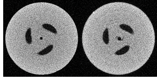
Figure 13. Neutron CT slice of the constrictor with surrounding cooling channels of Nozzle 1. Left: Prior to operation, right: after operation [21].
