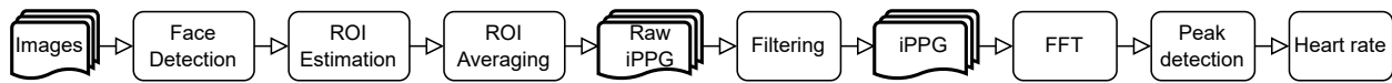
FIG 4. Processing pipeline for estimating the iPPG signal from a stream of camera images.
