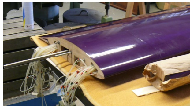
FIG 6. Root of the wing model with pressure hoses
