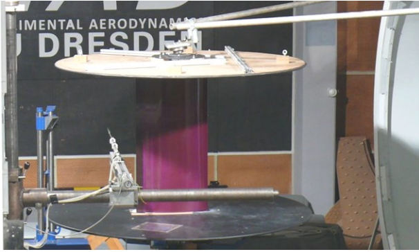
FIG 7. Wing model installed into the wind tunnel's test section
