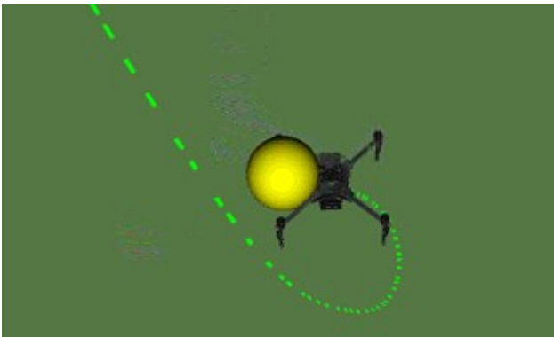
Figure 9: UAV overshooting the goal point (yellow). The green dotted line represents the flight path.
