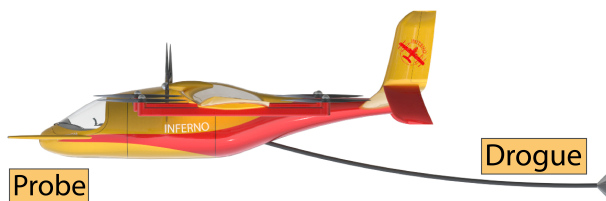
FIG 12. Drogue-and-probe concept for aerial refueling and maximizing firefighting time
