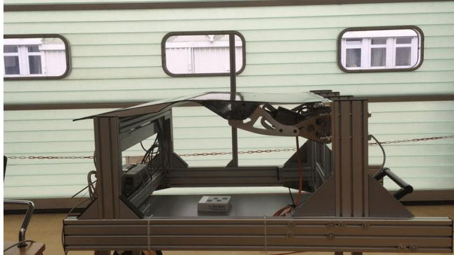
CRT functional demonstrator for spoiler with flexible hinge for laminar wing application
