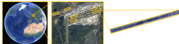
FIG. 1: Process of an airport localization, arrival runways identification, and touchdown zone extraction
