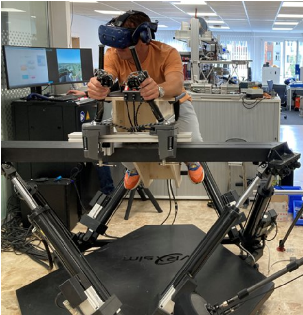
Fig. 21: 6DOF simulator platform to test the flight-controller software, vehicle control and seating.
