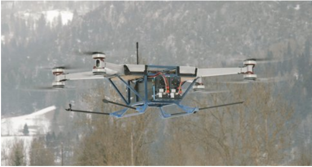
Fig. 20: IRON BIRD in hover-flight for performance test and data-logging of relevant data for post-processing.
