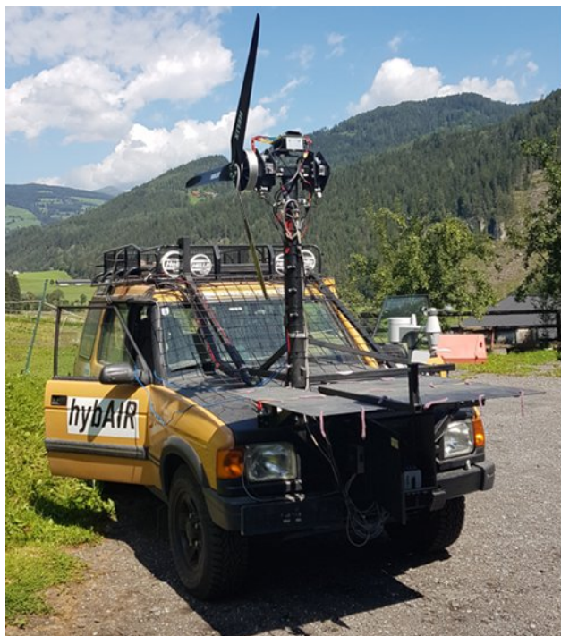
Fig. 17: Measurement setup for propeller performance tests on a pick-up truck as moving test platform.
