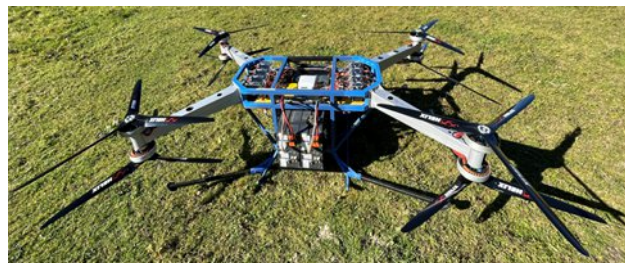
Fig.19: IRON BIRD demonstrator with target propellers, motors, inverters, boardcomputer and flight-controller software.
