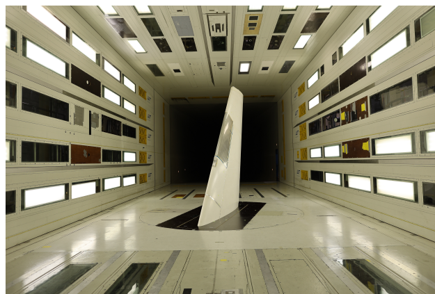
FIG 3. The VTP model in the test section of DNW-LLF, shown here with large sideslip angle for artistic reasons (Photo credits: DNW-LLF)
