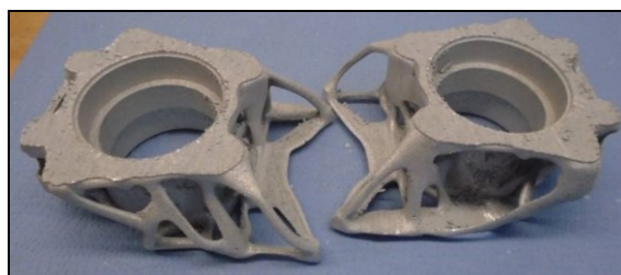
FIGURE 13. AM component Flange after additive manufacturing
