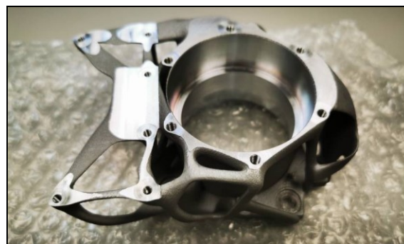
FIGURE 14. AM component Flange with post-processing during incoming inspection
