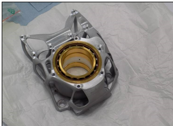
FIGURE 15. Partial assembly AM subassembly Flange
