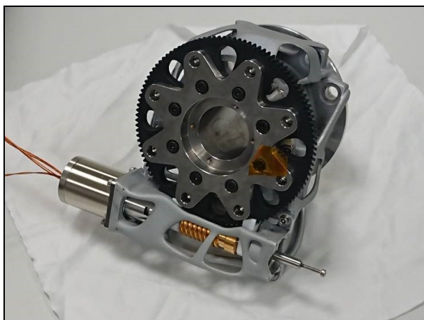
FIGURE 16. AM mechanism demonstrator after final assembly
