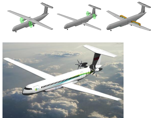
FIGURE 3. Three initial configurations for the SE 2 A short-range aircraft (top) and the final design (bottom)
