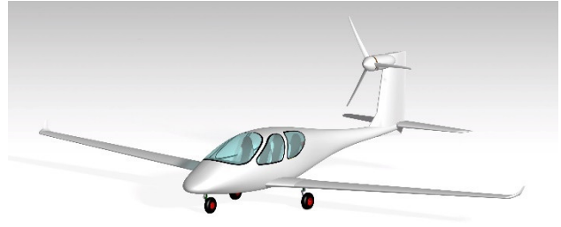
FIG. 2: Series hybrid-electric aircraft in CS-23 class: electric motor installed in vertical tail, combustion engine with generator integrated in the nose cone, battery system installed behind passengers [8]
