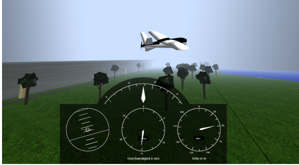
Figure 3: Illustration of the Web-Based Virtual Flight Test Environment.
