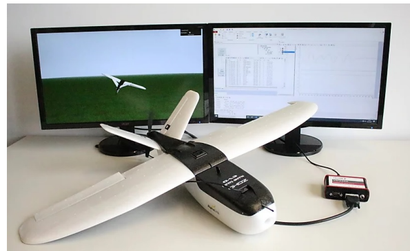
Figure 2: Hardware-in-the-Loop Simulator for ZOHD Nano Talon.
