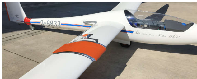
FIGURE 15 "Wing glove" mounted at the right wing of the Discus-2c
