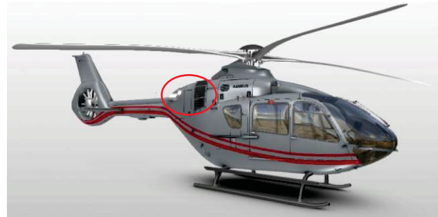
Figure 1: H135, typical small twin-engine helicopter with integrated engine design. Engine position marked with a red circle. Picture based on [1].
