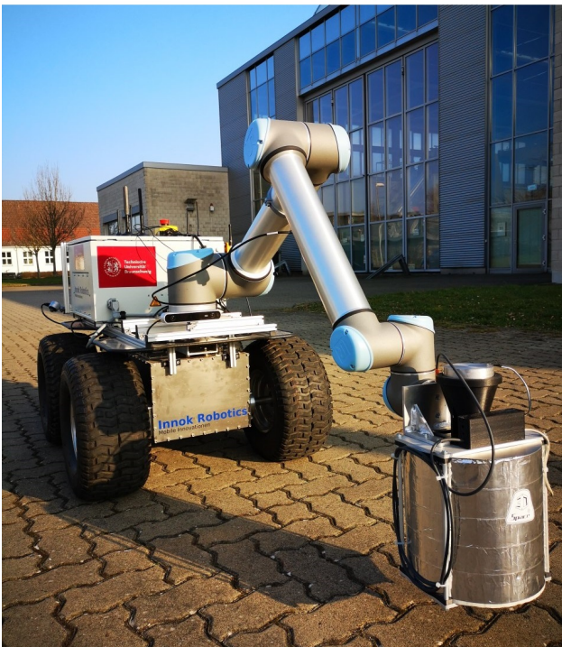
Figure 1: MIRA3D with a kinematic printhead dummy to test the robots behaviour with end-effector
