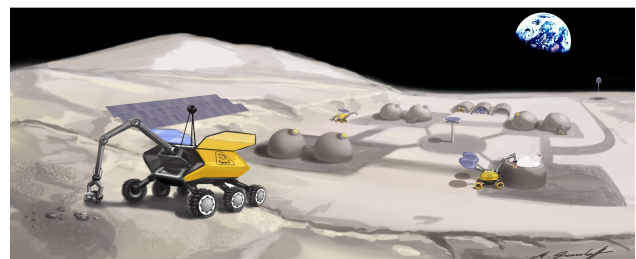
Figure 6: Artistic representation of the robots collecting and processing lunar regolith for habitats of a moon village. (Michael Grasshoff, ITD)
