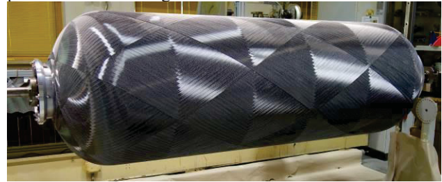
Figure 18: Dry carbon fiber preform of the booster casing containing the fiber optic sensors
