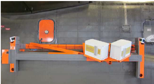
FIG 3. Sensor System Mounted on the Test Helicopter
