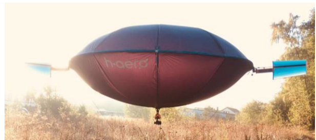
Image 7 Outdoor LTA UAV for industrial inspection needs with payload (b.II)
