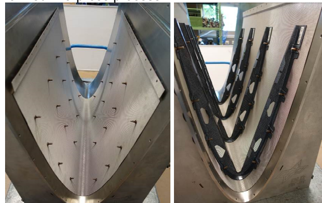
Figure 14: Formed outer skin with welded screws (left), stiffener ribs in formed outer skin (right)
