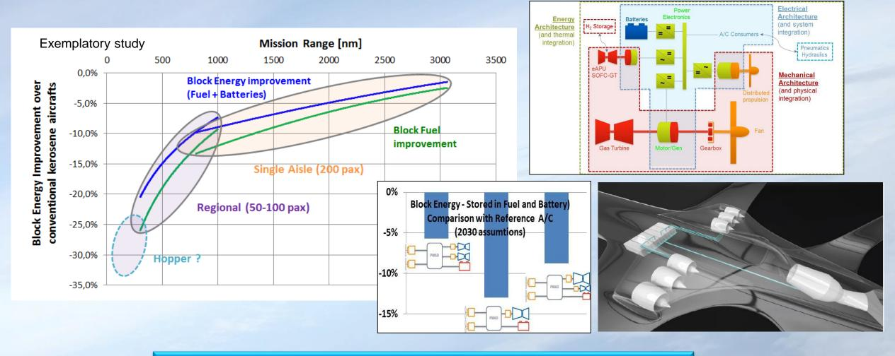
Hybrid / Electric propulsion can visibly reduce block energy need → but is this enough for a paradigm shift ?
