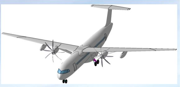
A very high aspect ratio wing can enable ultimate aerodynamic efficiency, but active control technologies and disruptive structural solutions are required
