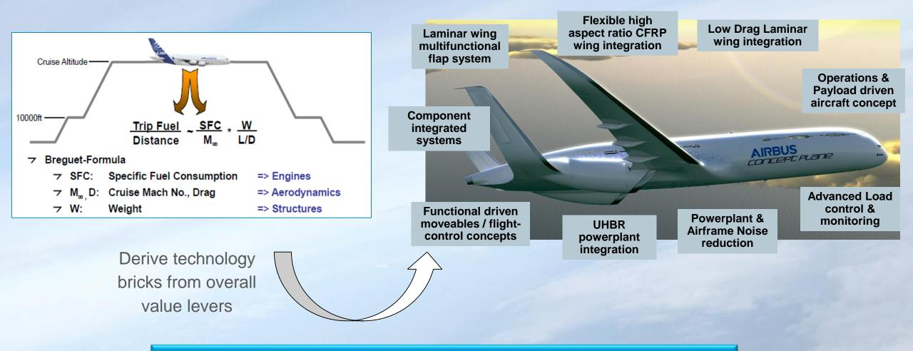
A key challenge is to ensure integration of novel component "technology bricks" to ensure overall level benefits maturing on aircraft level.
