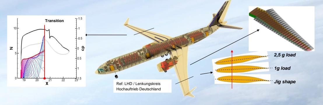
Optimized Laminar wing integration via change in wing planform design paradigms, enabled by advanced structural technology
