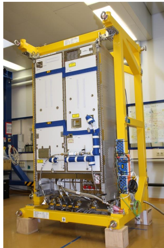
Fig. 1: ACLS – The Life Support Rack
