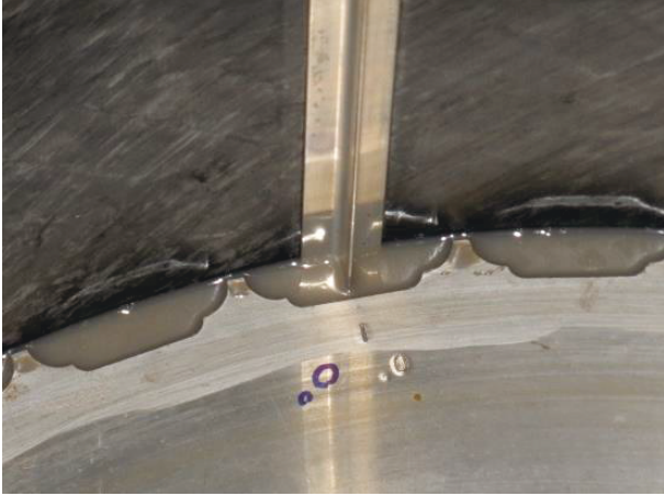
FIGURE 7. Potting of the specimen into the load introduction elements
