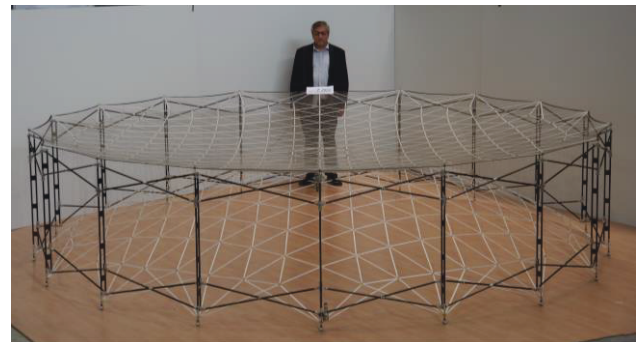
Figure 11. 5 m diameter reflector demonstrator with FlexRS-II technology for medium and large sizes and up to X-band of frequencies
