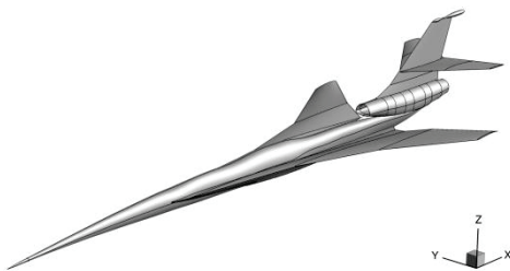
FIG 1. Geometry of the NASA C25D case with flow-through nacelle provided by the second AIAA Sonic Boom Prediction Workshop
