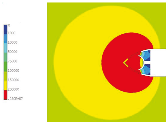
Fig. 2: 2D electrostatic field around the radome area in a 100 kV/m ambient electric field.
