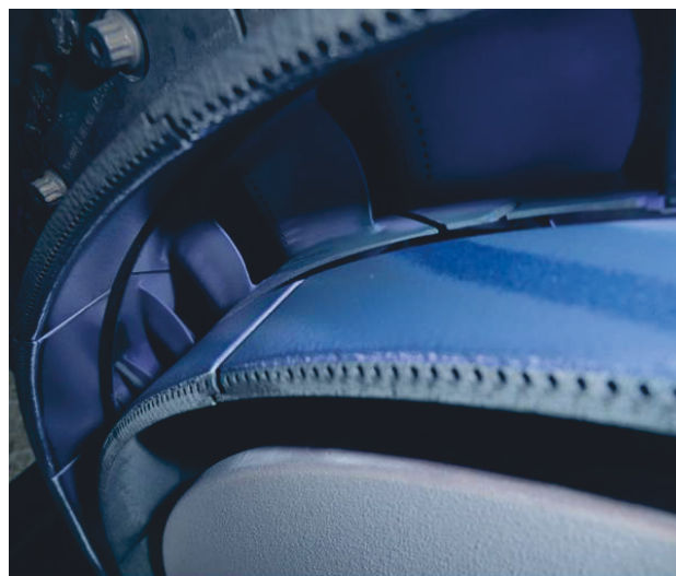
Figure 13: Thermal paint snapshot after test
