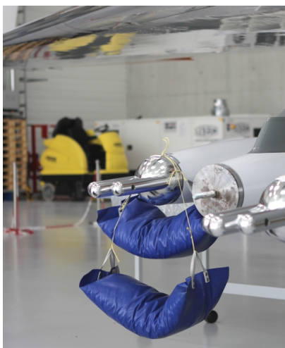
FIGURE 15. Strain gage calibration for one PMS carrier
