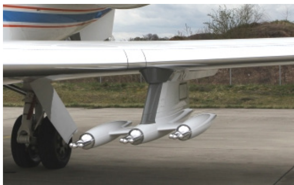
FIGURE 11. PMS carrier mounted on the wing station
