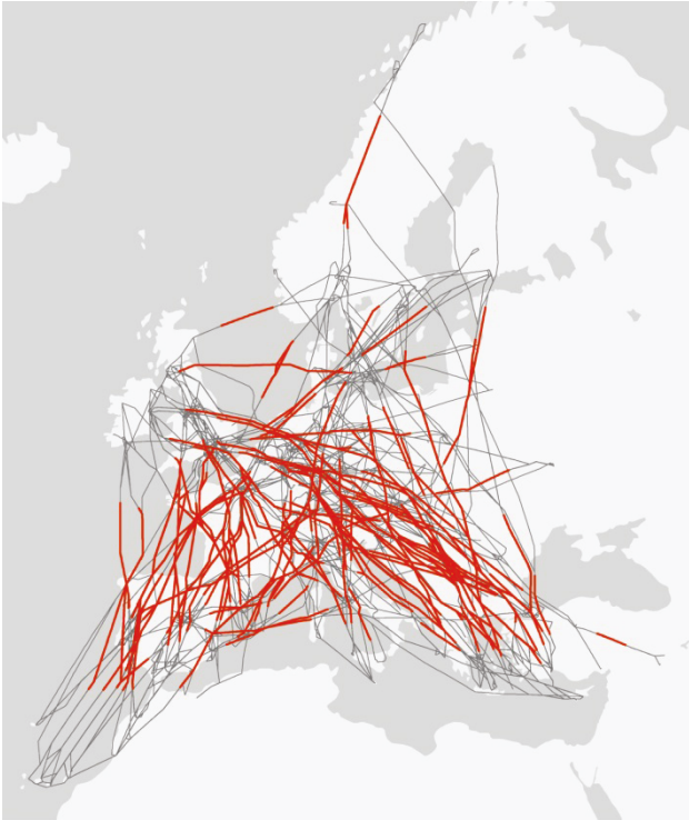
FIG 2. Ground tracks of identified formation missions with resulting formation segments colored in red, other segments in gray
