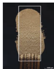
FIGURE 11. Cladded volume on a flat substrate
