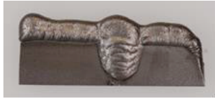
FIGURE 12. Crack and volume cladding
