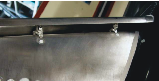
FIG. 12. Slat tracks and pressure tube bundles on the DLR-F11 high lift configuration, view from below.
