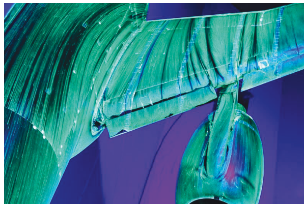
FIG. 20. Oil flow visualization for the JAXA JSM high lift configuration
