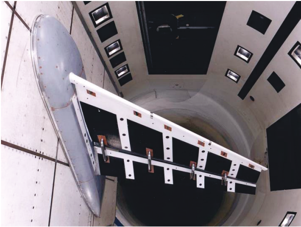
FIG. 1. NASA Trap Wing in the 14 x 22 wind tunnel of NASA LaRC
