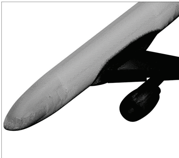
FIG. 21. SOLAR surface grid for the JAXA JSM high lift configuration on the medium grid level
