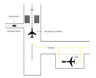
FIGURE 3. Aerodrome concept line-up with "Engine-Start-Area" (ESA) for RPA [9]
