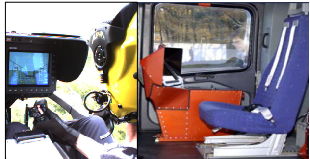
Figure 12: Evaluation pilot (EP) during the trial following the flight path with a Tunnel-in-the-sky instrument and flight test engineer workstation
