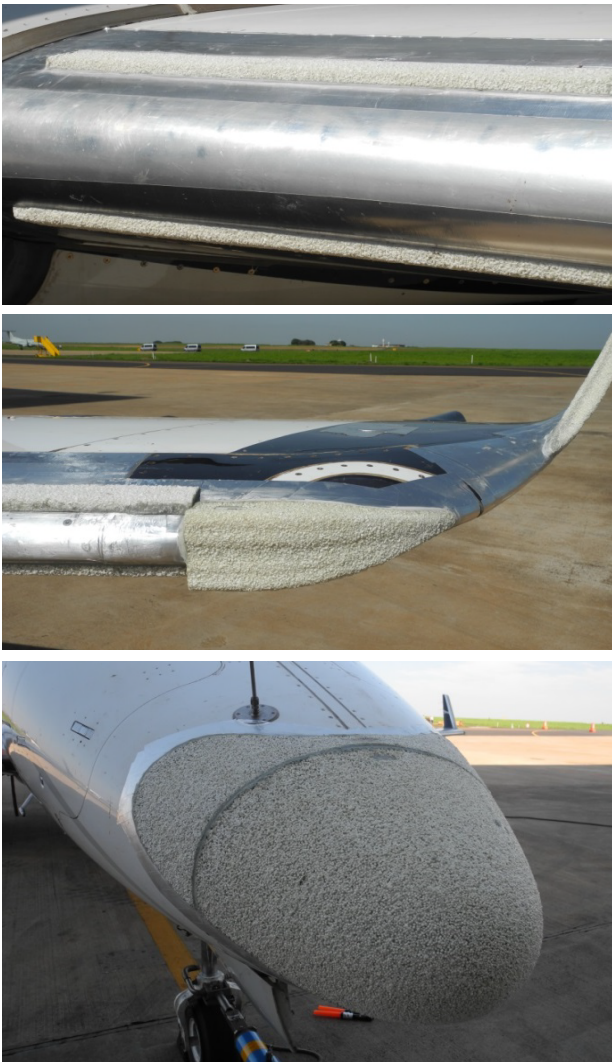
Figure 8: Artificial shapes for SLD icing on the upper and lower wing surface, outer wing and radome.
