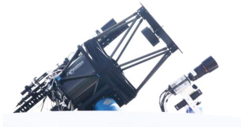
Figure 1: Stare and Chase assembly: The staring camera is used for initial detection of RSOs, while the telescope recaptures the detected objects for precise measurements.
