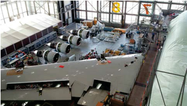
Bild 9. SOFIA in Dock, engines removed (left).
