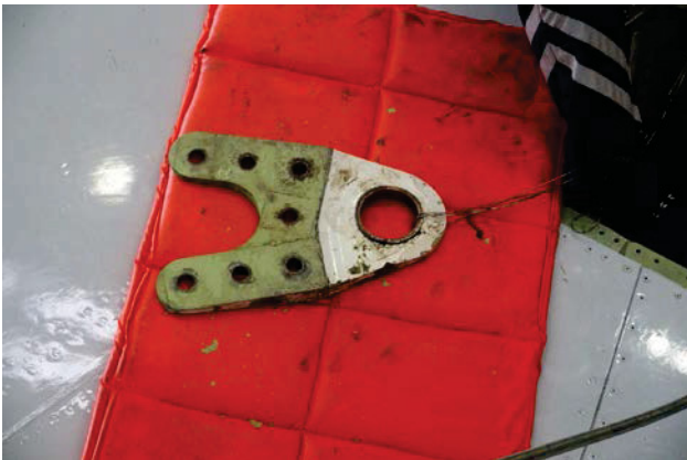
Bild 12. RH wing gear support end fitting removed.
