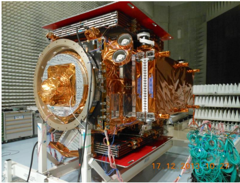
LCT – successful integrated and tested on Sentinel 1A (Dez 2013)
