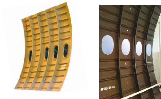
Fig. 1: Fuselage mock-ups for an Al- based (left) and CFRP based (right) design concept
