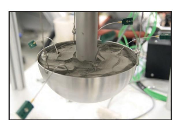
Lunar regolith heating and gas extraction experiments Sample transport experimentats on partial-g parabolic flight
