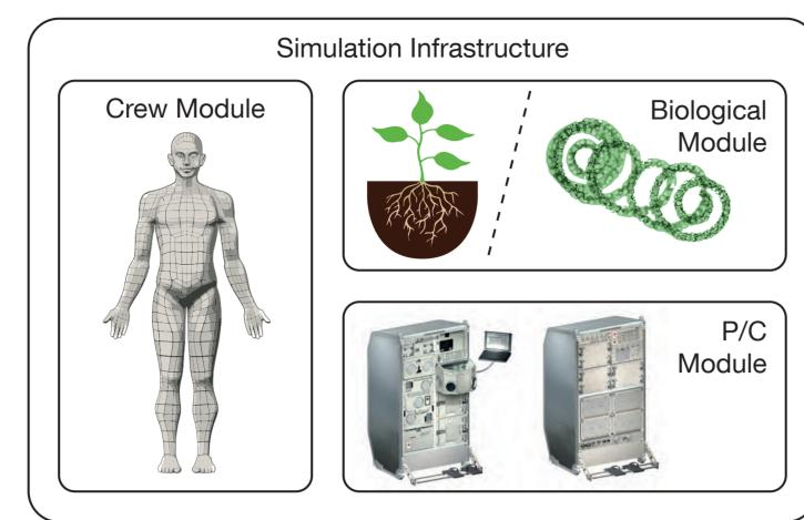
applications in closed environments. Using a set of intelligent, variable time step solvers, a wide variety of physical, chemical and biological effects can be simulated. V-HAB also includes a dynamic human physiology model to provide realistic inputs to the LSS.
