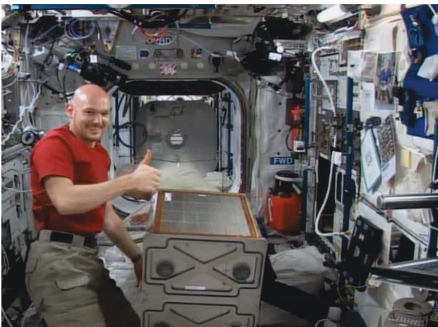
FIG. 4. German Astronaut Alexander Gerst working on the installation of the EML Experiment Module into the EDR Rack on board the ISS
