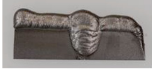
FIGURE 12. Crack and volume cladding
