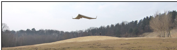
FIGURE 26. First flight of the Flying V (28.02.2014, Berlin, Germany): The model was thrown from a little hill out of a height of roughly 3.5m. After a short and fast decent to gain speed after the throw a straight glide path could be taken up on which the Flying V flew roughly 90m. The airplane was easy to control and landed smoothly.
