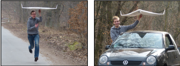
FIGURE 25. The glider model weighs 770g and has a wing area of 0.43\text{m}^2 . To achieve the design C_L=0.25 a speed of roughly 40km/h is required. After first slower tests with running the model was brought up to 40km/h with a car. The rudders were tested and the model seemed well trimmed for a neutral flap position at this speed and stable.
